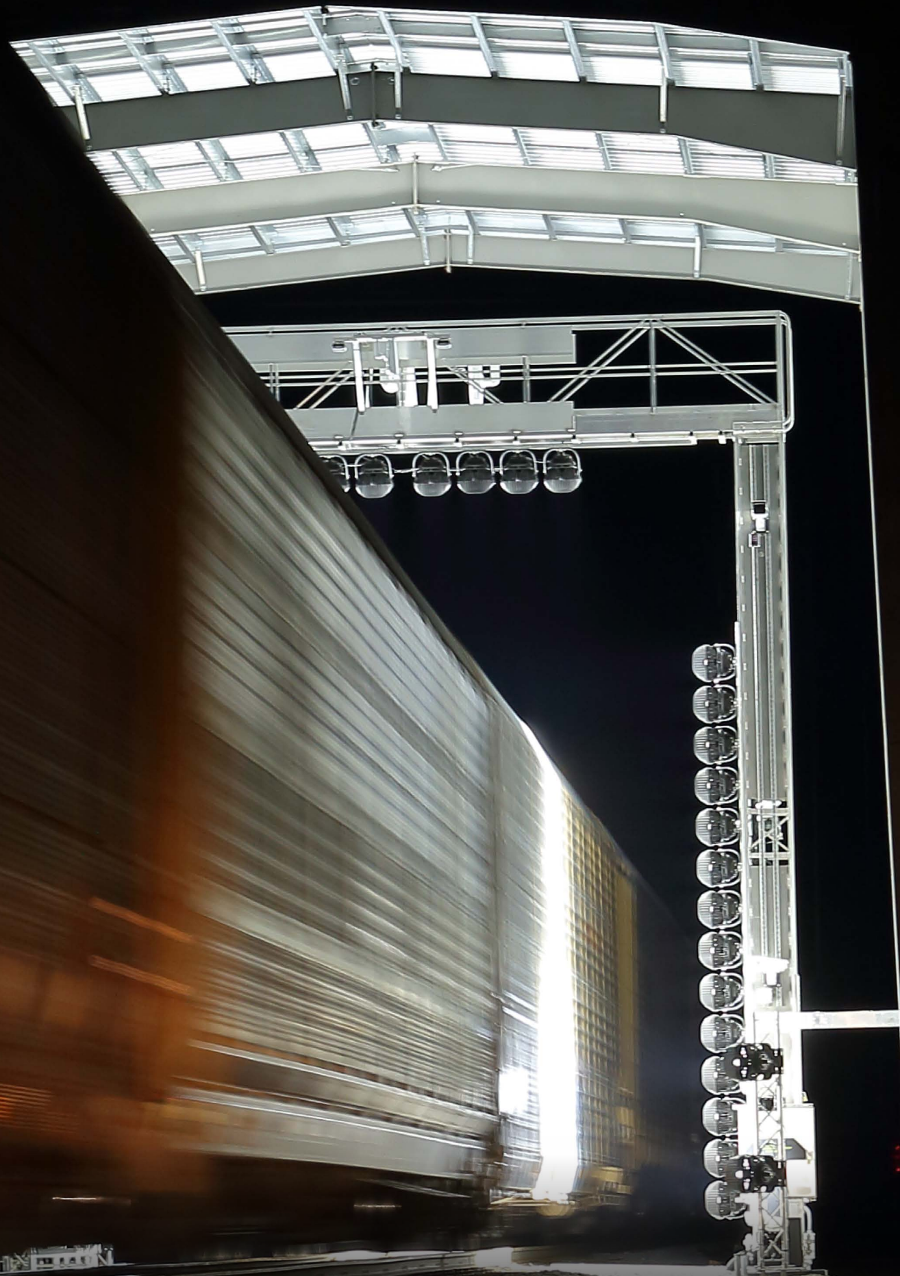
17 ultra-high definition cameras scan trains at rail speed. <<
